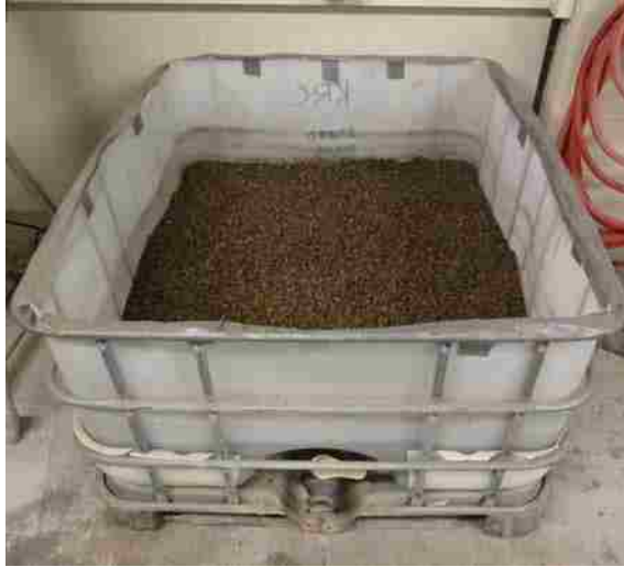
Figure 3.3 Tank Used for Lightweight Aggregate Saturation
