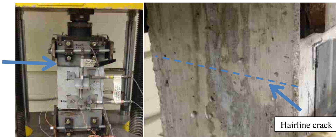
Figure 3.20 Location and Example of Hairline Flexural Cracks
