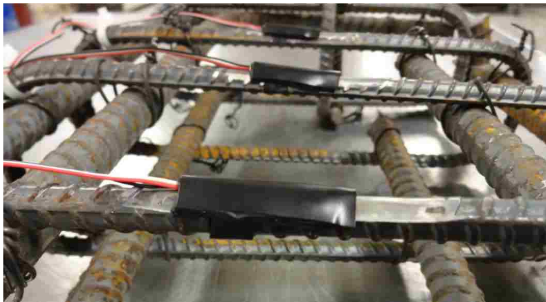
Figure 3.19 Strain Gages Attached to Shear Reinforcement
