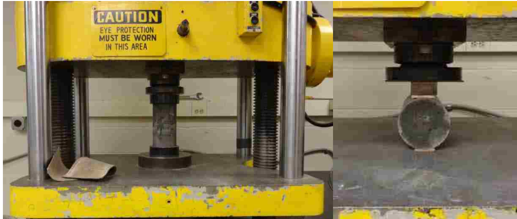
Figure 3.6 Cylinder Compressive Strength Test (left), Splitting Tensile Strength Test (right)
