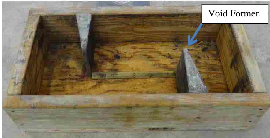
Figure 3.10 Formwork for Specimens with a Monolithic Interface
