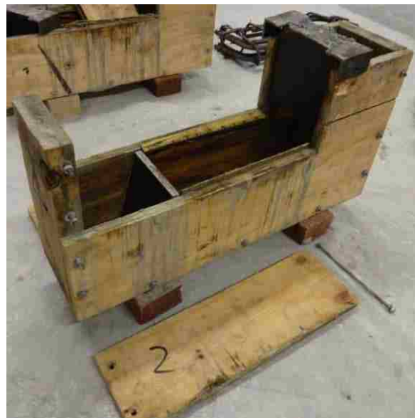
Figure 3.11 Formwork for Specimens with a Cold Joint Interface
