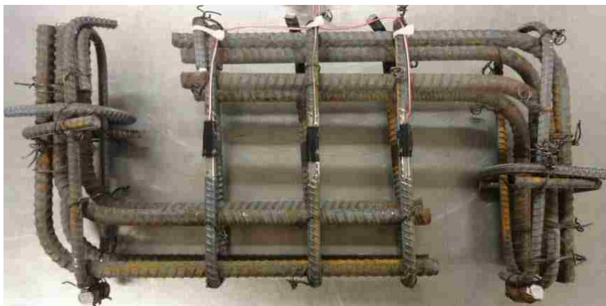
Figure 3.9 Reinforcement Cage with Strain Gages
