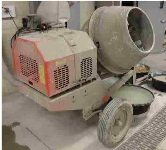
Figure 3.4 Six Cubic Foot Rotary Drum Mixer
