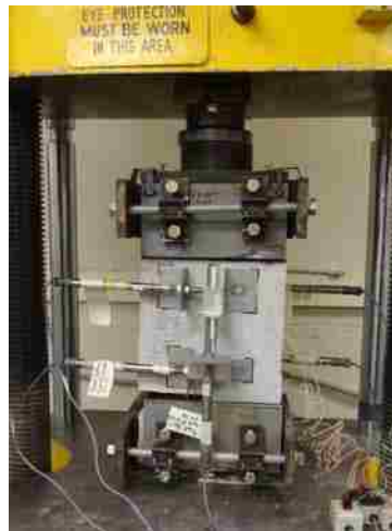
Figure 3.14 Typical Support Conditions for Testing
