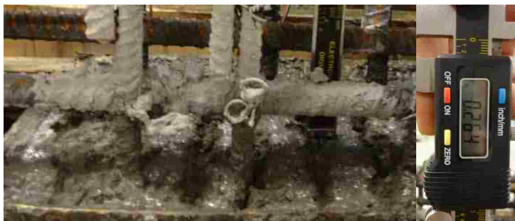
Figure 3.13 Example of Roughened Surface and Measuring of Roughness
